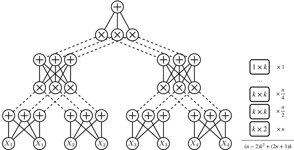
(a) We show the structure of a RAT-SPN over  $n = 4$  variables using layer size  $k = 3$ . Solid edges are weighted with trainable parameters, and dashed edges are unweighted. Each fully connected layer of solid edges can be treated as a sector.
