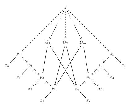
Figure 4: A decomposable circuit g constructed based on input intervals. Edges are solid if the parent is a  $\otimes$ -gate, and edges are dashed if the parent is a  $\oplus$ -gate. In this example the input intervals are  $\{[3,3],[2,3],[2,2]\}$ .
